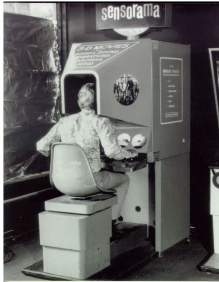
(b) The Sensorama, created by Morton Heilig, which used a stereoscopic movie, binaural sound and a fan to create an immersive VR experience. [Afn]
