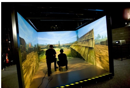
(c) The CAVE system, developed by Cruz-Neira et al. Polarized light is projected onto all six sides of the cuboid the user is located in. [Afn]
